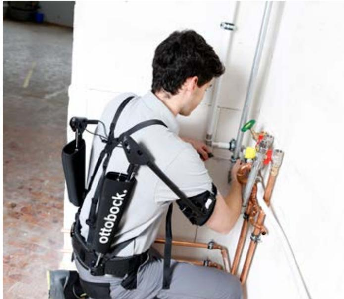
The Paexo Shoulder exoskeleton assists employees in production and construction during strenuous activities, in particular overhead work. The raised arms are held up by an innovative expander technology. This provides noticeable relief for the muscles and joints in the shoulder region. Overhead activities are much more comfortable to perform.
